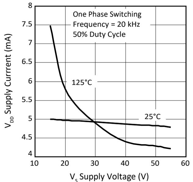
Figure 7:  $V_{DD}$  消費電流
